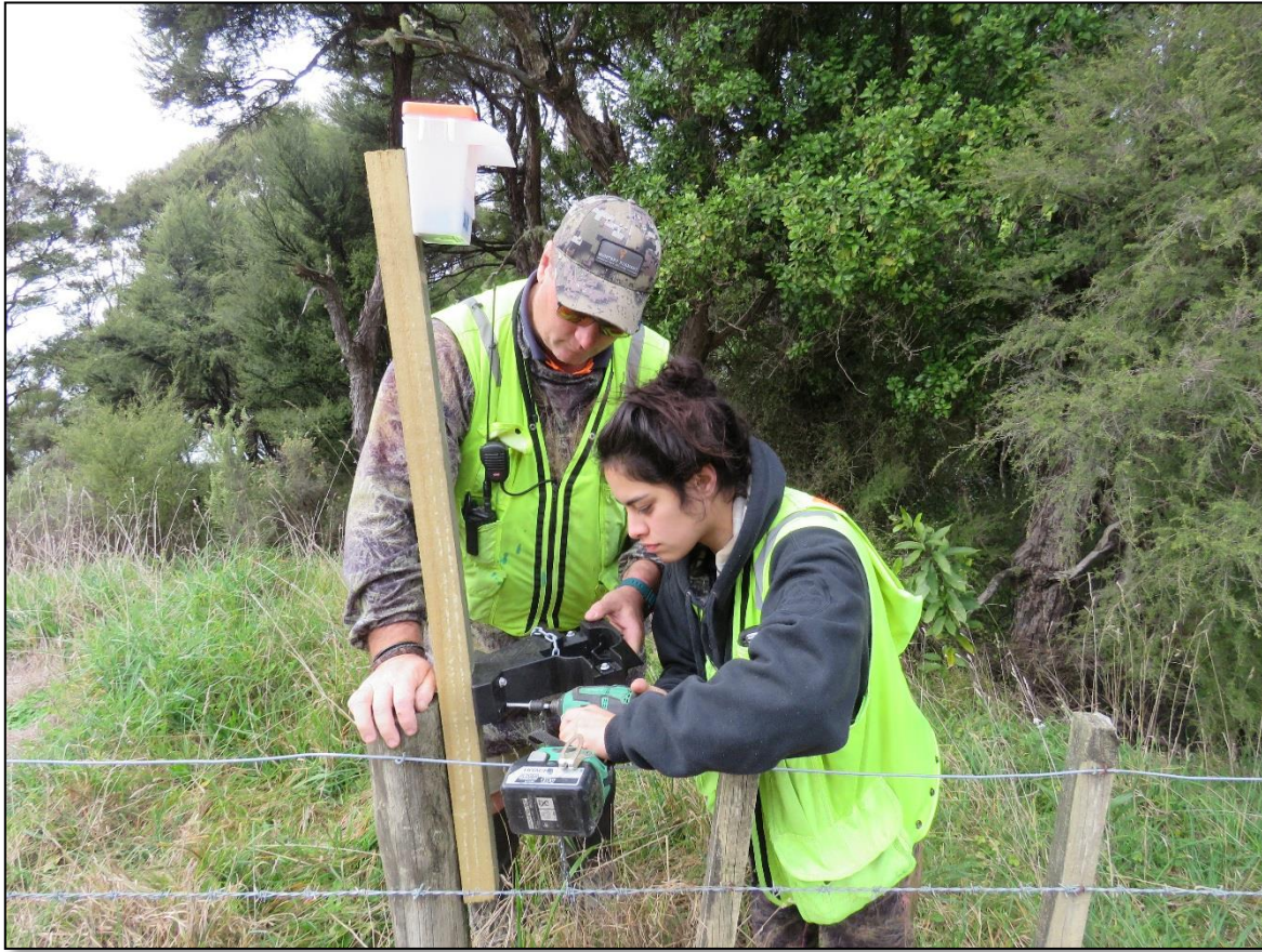
Michaela King-Peters and Shane Diphoom installing a wirelessly monitored leghold trap.
